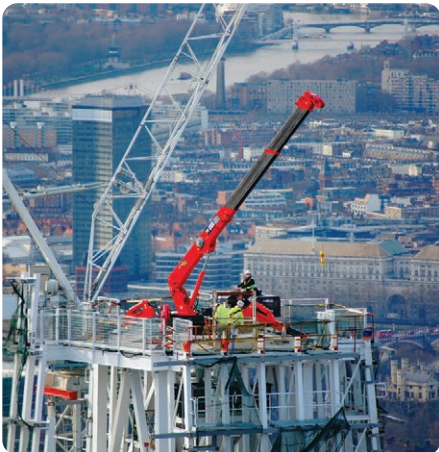
Fly Jib - 800kg Maximum Capacity
