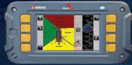
Optional Variable Footprint safe load indicator
