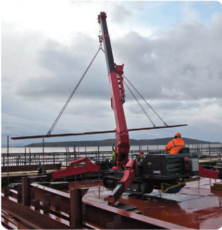
Searcher Hook - 800kg Maximum Capacity
