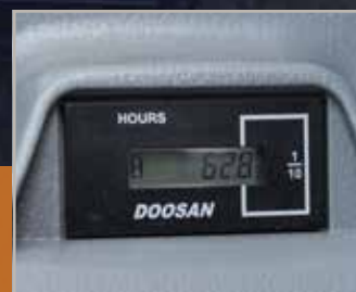
Hour meter (from ground level)
